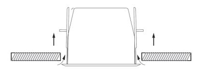
Step 2: loose the metal plates and rise them up to the top. Insert the back can into the mounting hole.
