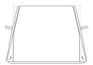
Step 1: measure the mounting hole. It must be as the cutout size of the device. Pass the cable through the cable gland.
