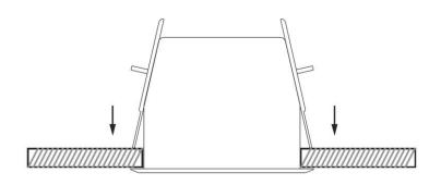
Step 3: slide down the metal plates until they reach the surface. Tight the fasteners inside the back can.
