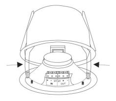
Step 4: connect the audio cable to the loudspeaker's terminal block. Finally, insert the mounting springs into the hooks and push the loudspeaker into the back can.
